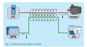
As soon as an electrical conductor is exposed to a changing magnetic field induction will result. In this instance, this results in a shield current on the bus line.
