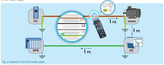
A prerequisite to keep the above described problems under control consists in using symmetrical motor lines combined with professional expert installation of an adequate earthing and equipotential bonding system.
