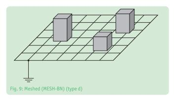
Generally, all devices in the control cabinet need to be arranged and wired as EMC-compatible. This includes all FE/BN connections of electrical equipment being integrated with low impedance and shortest possible distance into the bonding of the electrical cabinets (rear wall and main bonding rail). The same
