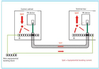
Fig. 16: Function 2 – Additional functional bonding
