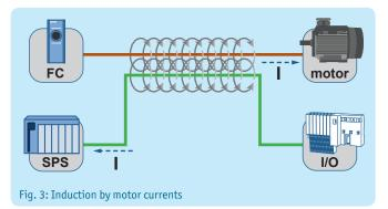
As soon as an electrical conductor is exposed to a changing magnetic field induction will result. In this instance, this results in a shield current on the bus line.
