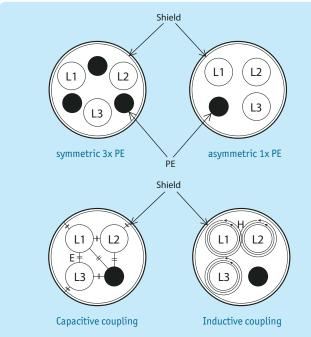
Fig. 17: Couplings, asymmetric motor cable
