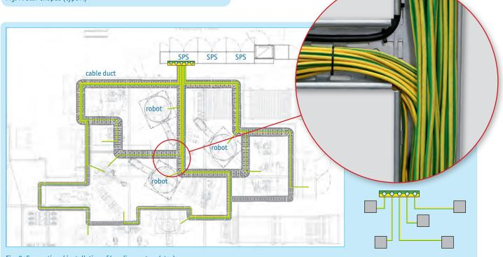
Fig. 8: Conventional installation of bonding system (star)
