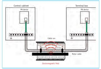
Fig. 15: Function 1 – Additional shield in environment with heavy field load
