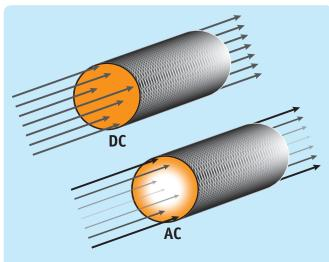
Fig. 11: Skin effect for direct and alternating current
