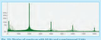
Fig. 23: Display of spectrum with 50 Hz and superimposed 2 kHz
