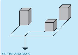
Compared to a strongly meshed bonding system (MESH-BN, see right side) the star-shaped arrangement provides only very few flow paths for compensating currents resulting in heavy loads on the bonding system and the central earthing point. Often long distances need to be bridged to connect devices what results in high installation costs.
