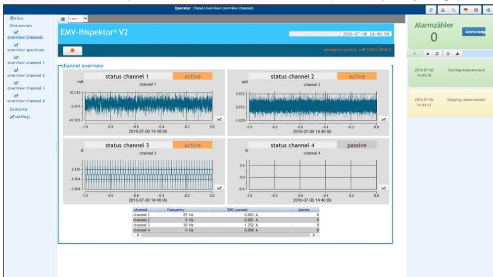
The "channel overview" provides information on the present current course, the corresponding effective value, the main frequency, and the number of alarms for each channel.
