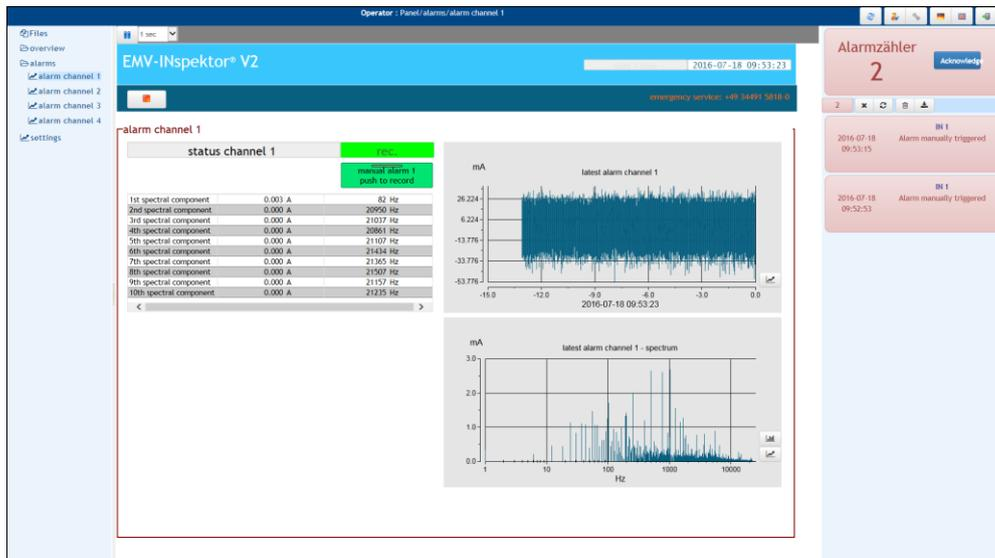
The alarm overview first displays the data record that was last saved (current course & frequency spectrum per channel), provided that a previously set trigger was fired. In addition, the corresponding current and frequency values of the 10 largest spectral components are listed as a table. The "manual alarm" button allows spontaneous recording of current actual values (e.g. for documentation purposes).
