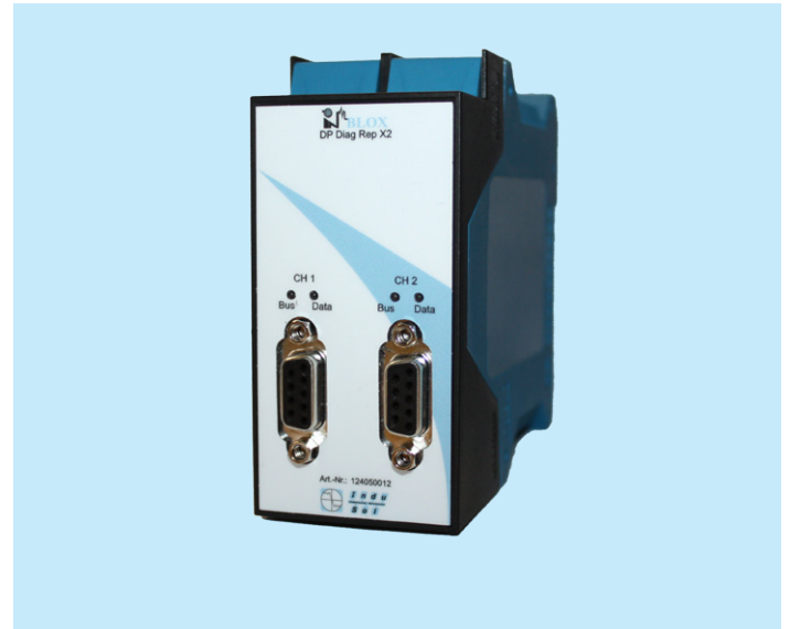
INBLOX® Extension module Diag Rep X2
