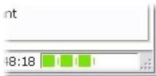
Additionally the standard elements for the 'Windows' windows are available, eg. the buttons in the top right hand corner. Furthermore, a handle in the lower right hand corner is available, with which the window can be pulled to the desired size. The minimum size is 600x800 pixel. The maximum size is limited to 1000x1400 pixel, but may also depend on the monitor size and its resolution.
