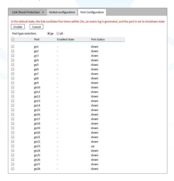
The main element configuration description of port configuration interface:
