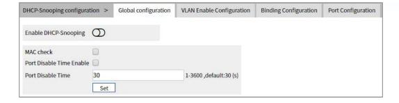
The main element configuration description of global configuration interface:
