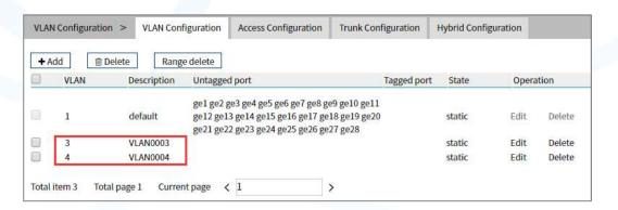
**Step 3** Set the corresponding pvid of port3 and port4, as well as the type of port2, port 3 and port4.
