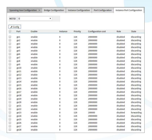
The main element configuration description of instance port configuration interface:
