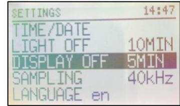
While recording or observing a current, the clamp will switch into standby mode after the set time.
