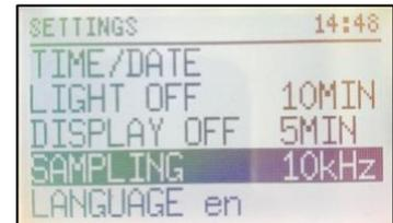
Changing the sampling frequency also changes the measurable frequency range. The sampling frequency should always feature at least the double value of the frequency to be measured. The higher the sampling frequency, the shorter the battery life.
