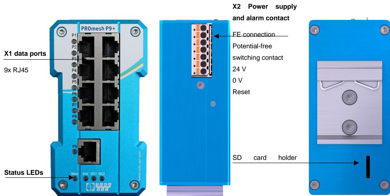
Figure 1: Device connections
