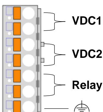
Figure 4: Connector terminal block assignment
