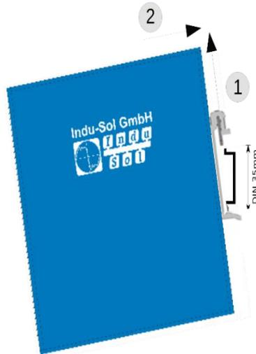
Figure 3: Mounting and dismounting on the top-hat rail
