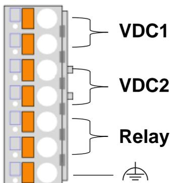
Figure 4: Connector terminal block assignment
