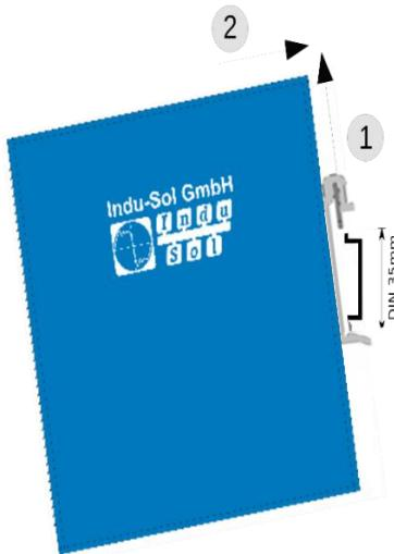
Figure 3: Mounting and dismounting on the top-hat rail
