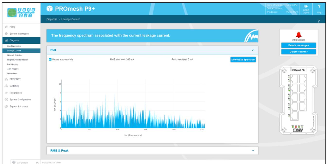
Figure 11: Leakage current
