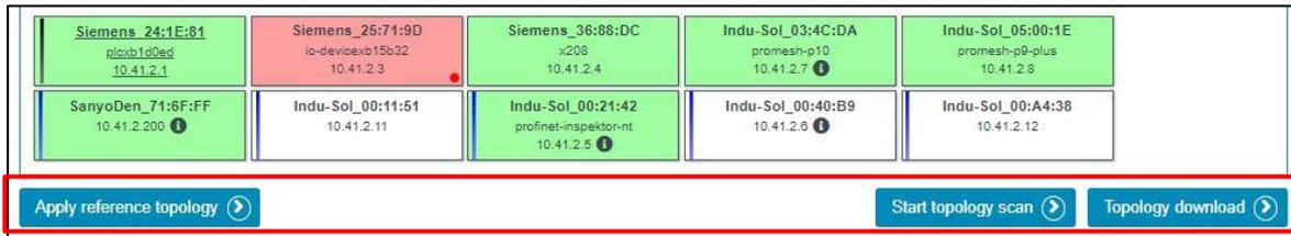
Figure 137: Determination of the reference topology
