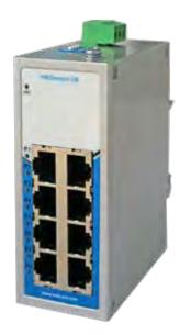
**Unmanaged Switches** are the simplest and most costeffective type of network switches. They are ideal for small networks where no configuration is required, offering a plug-and-play solution. These switches are excellent for simple applications where no network traffic management or specific security or performance requirements exist. For longterm disturbance-free and maintenance-friendly operation, managed switches are generally recommended.
